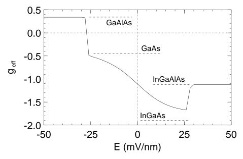
Figure 2. The effective g-factor  $g_{\rm eff}$  of electrons confined in a  ${\rm Ga_{1-x}Al_xAs}$  -  ${\rm GaAs}$  -  ${\rm Ga_{1-y}In_yAs}$  -  ${\rm Ga_{1-x-y}Al_xIn_yAs}$  heterostructure  $(x=0.3,\ y=0.1)$  as a function of the applied electric field E in growth direction. The widths of the quantum well and the barriers are  $w=w_{\rm B}=10\,{\rm nm}$ . The g-factors which are used for the materials are indicated with horizontal lines.
