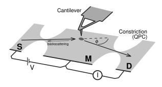
FIG. 1. The proposed setup. An applied bias voltage V between the source S and the middle region M injects a current into the graphene sheet. The injected electrons scatter from an artificial scatterer created by a SPM tip above the surface. The flux of electrons that are coherently scattered into the drain D can be detected in the drain current I.
