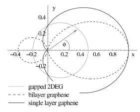
FIG. 3. Differential cross section normalized by  $2\pi(kR)^4(U_0/E)^2$  in units of 1/k for a circular scatterer of the Gaussian shape. For single layer graphene, the Berry phase of  $\pi$  prohibits backscattering, while for bilayer graphene, the Berry phase of  $2\pi$  prohibits rectangular deflection. The radius of the scatterer is chosen kR=0.5 for this plot.
