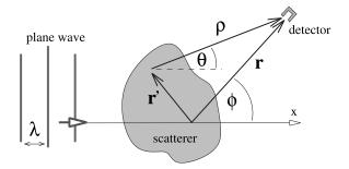
FIG. 2. Formulation of the scattering problem: an incoming plane wave propagating along the x direction hits the scattering potential. A detector measures the outgoing flux of the scattered wave as a function of the deflection angle  $\phi$ .
